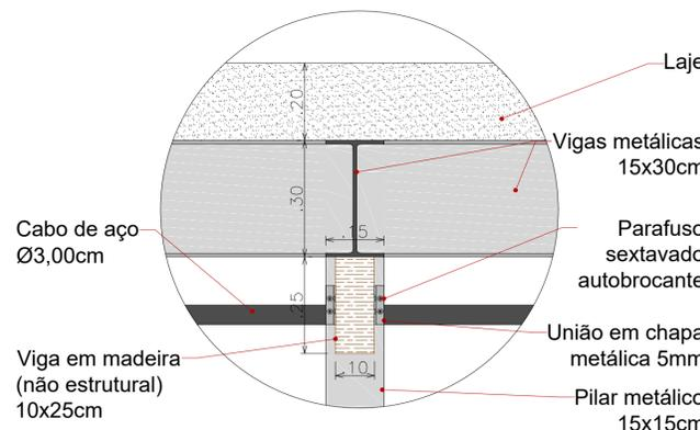
DETALHE 04 - CORTE TRANSVERSAL APOIO VIGA MADEIRA | ESCALA 1:10
