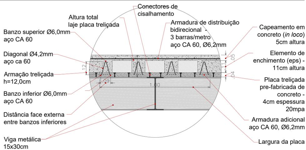
DETALHE 02 - CORTE LONGITUDINAL LAJE/APOIO VIGA | ESCALA 1:10
