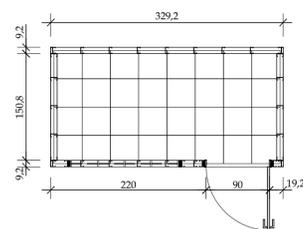
MALHA COM STEEL FRAME | ESCALA 1/50
