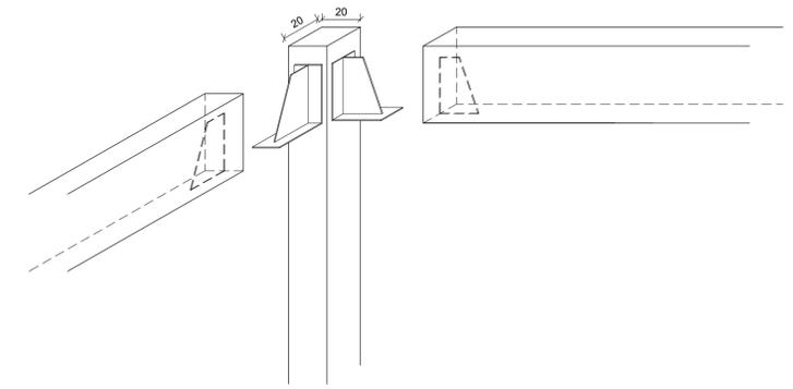
DETALHE JUNÇÃO VIGA/PILAR MLC
